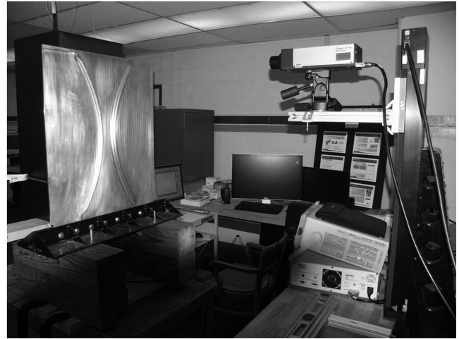
Fig. 7 Laser vibrometer and support equipment in place for testing.
